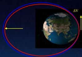
$$\epsilon_{orbit} = -\frac{\mu}{2a_{orbit}} = -\frac{\mu}{2a_{orbit0}} + \frac{\text{Energy added}}{m \text{ satellite}}$$
