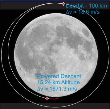
Landing begins with the LSAM in a 100 km circular orbit. A retrograde burn lowers perilune, and the lander coasts for half an orbit. Near perilune, powered descent begins, bringing the LSAM to a soft surface landing. Powered descent occurs in three phases:
