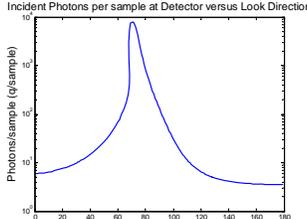
Expected photon flux incident on detector surface at various look angles (0° - 180°)
